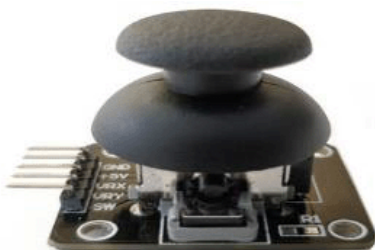
2-axis joystick with push button function
